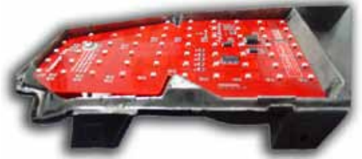
LED panels should sit flat and flush in the tail light housing.
